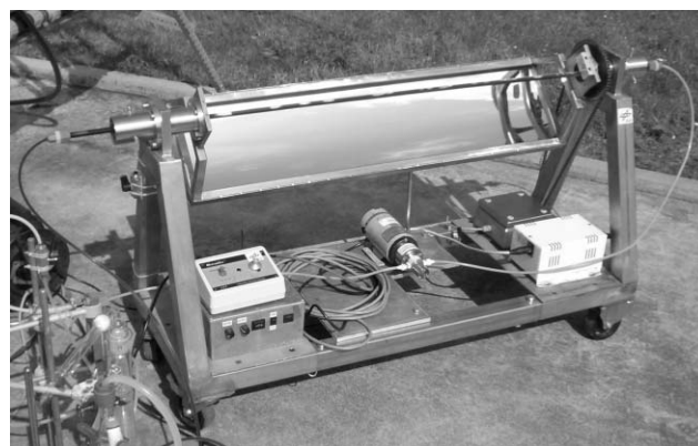
Fig. 1 Small-scale parabolic trough reactor equipped with aluminum mirrors. The storage vessel and O 2 -feeding equipment can be seen on the lower left hand-side.
