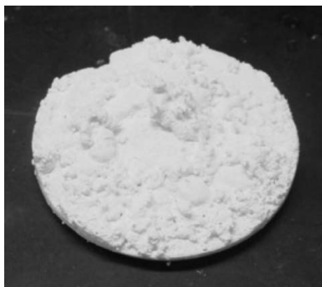
Fig. 2 A sample puck of PEG-1500 containing encapsulated RhCl(PPh 3 ) 3 .
